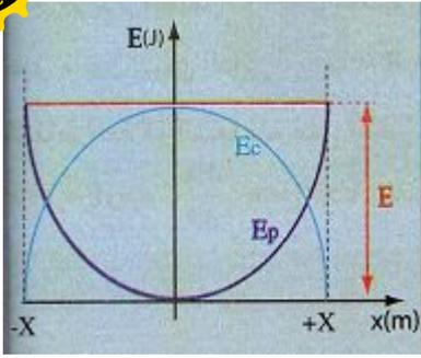
$$E = E_C + E_P , E_{pp} = 0 , E_{Pe} = \frac{1}{2} kx^2 , E_C = \frac{1}{2} m v^2$$
