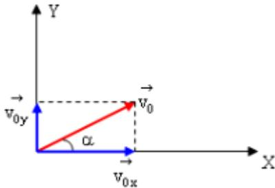
$$\text{tg} \alpha = \frac{v_{0y}}{v_{0x}} = \frac{4,10}{2,56} = 1,60 \longrightarrow \alpha = 58,02^\circ$$
